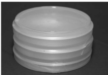
Plates stored agar side up, wrapped in parafilm.
